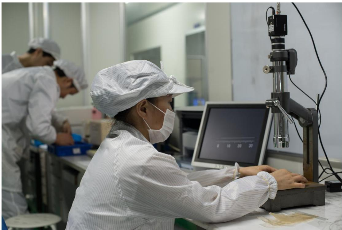
Collimator for testing cubes beam deviation
