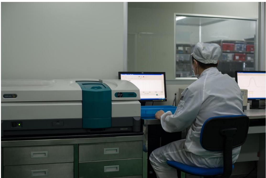
Cary 5000 Photospectrometer for measuring transmission, OD6 of blocking depth can be recognized
