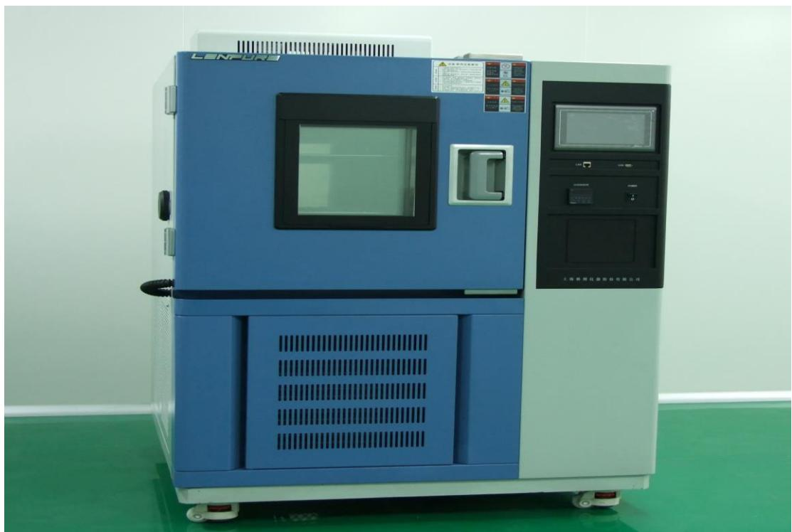
High Low Temperature and Humidity Testing
